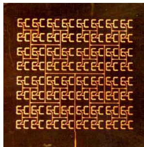
Fig. 3.6: 16x16 patch antenna array.
