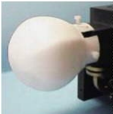
Fig. 4.5: Lens antenna (#1) operating at 58.5 GHz.
