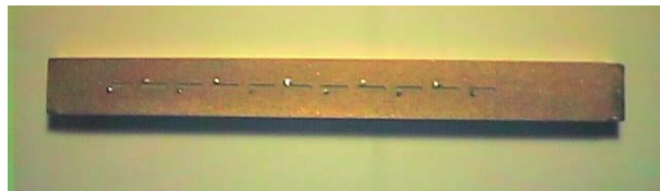
Fig. 2.7: Longitudinal slot waveguide Antenna fed by probe.
