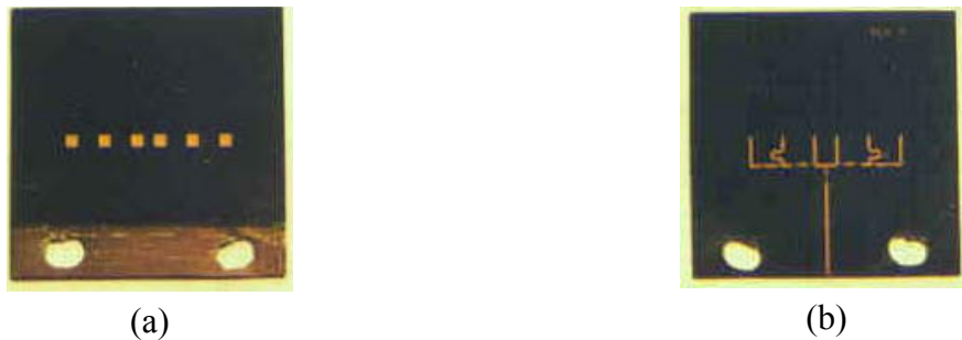
Fig. 3.4: Linear array. (a) Radiating elements (spacing between patches= 0,72 \times \lambda_0 , excepted between both central elements ( 0,5 \times \lambda_0 )). (b) Feeding network: Amplitude and phase taper: (0.15, 0^\circ) , (0.282, 180^\circ) , (1, 0^\circ) ; (1, 0^\circ) , (0.282, 180^\circ) , (0.15, 0^\circ) .
