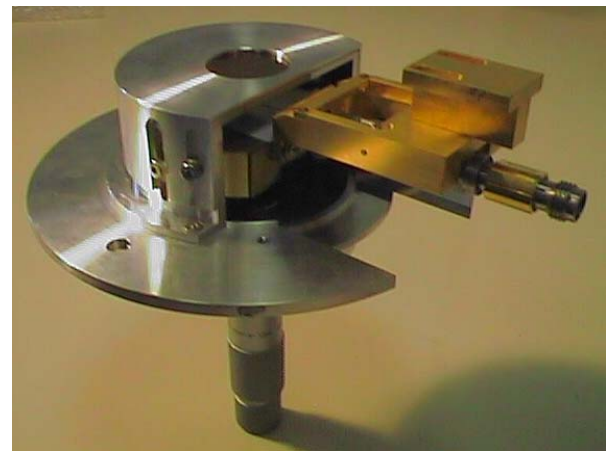
Fig. 5.11: Experimental setup for radiation patterns and gain measurements.
