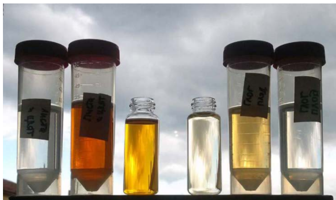
Figure 1: (from left) Hawthorn extract leaves & flowers (permeate, concentrate, feed); hawthorn extract fruit (feed, concentrate, permeate).
