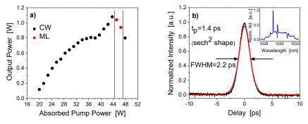
Figure 1: (a) Input-output characteristics of the laser in CW (black dots) and ML operation (red dots). (b) Autocorrelation curve (black line) and fit assuming sech2 pulse shape (red line); optical spectrum (inset).
